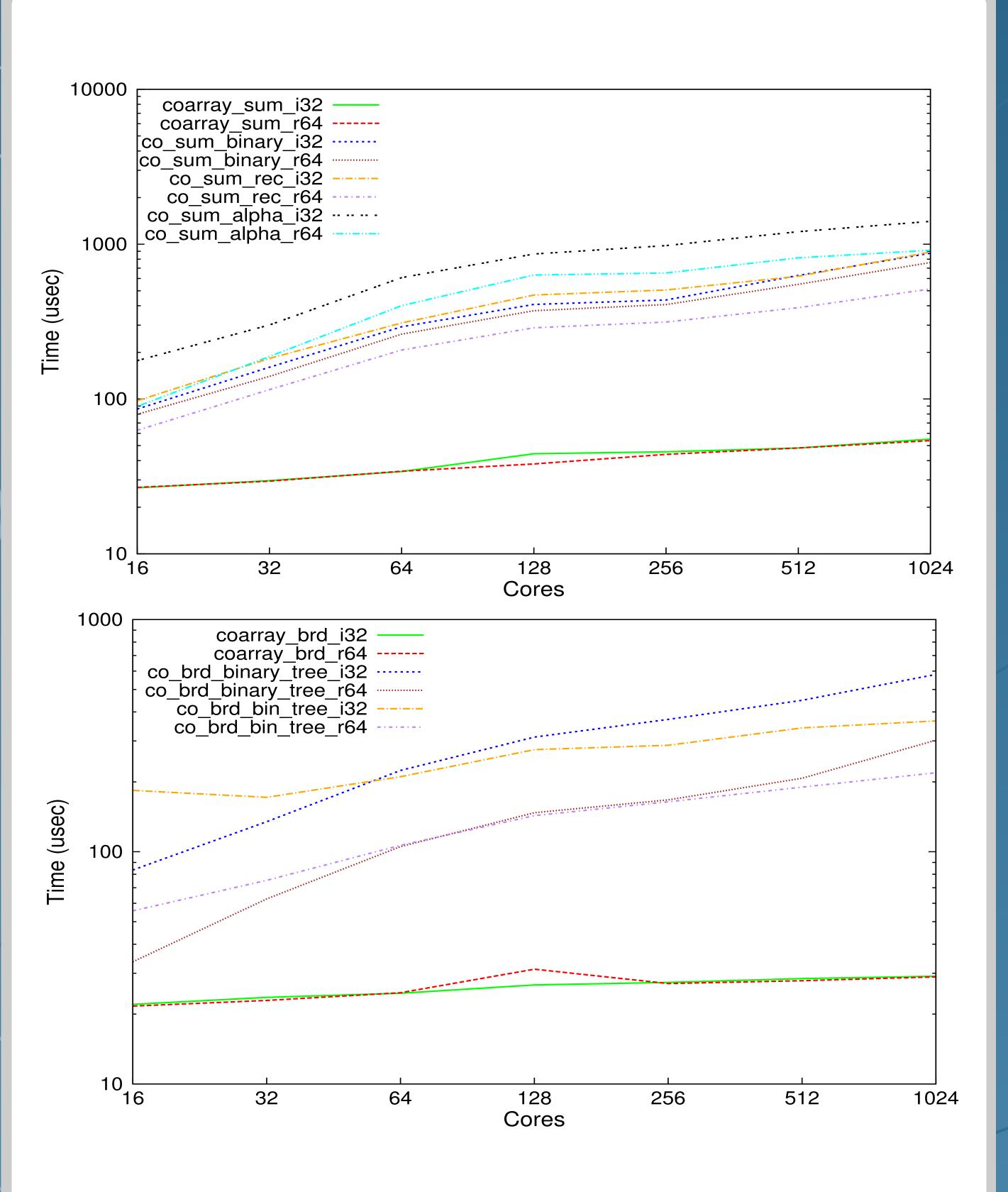
Execution times for sum reductions (top) and broadcasts (bottom). From top to bottom in the legend: intrinsics (red and green), binary tree, recursive doubling (binomial tree), and alpha tree (alpha=0.4). Platform: NERSC Hopper Cray XE6, peak performance of 1.28 Petaflops/sec, 153,216 compute cores, 212 Terabytes of memory, and 2 Petabytes of disk.
