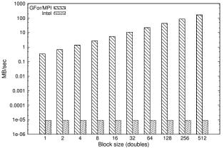
Figure 9: Bandwidth single Put on 2 compute nodes - Yellowstone 32 cores
