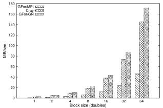
Figure 10: Bandwidth for small block sizes - Hopper 24 cores
