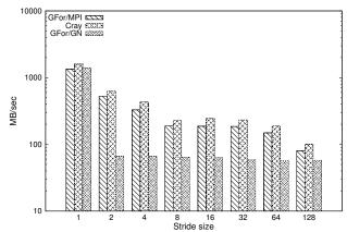
Figure 16: Strided Get on single node - Hopper 24 cores
