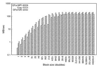
Figure 22: Bandwidth for multi pt2pt Get - Hopper 48 cores
