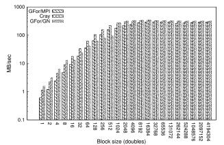
Figure 23: Bandwidth for multi pt2pt Get - Edison 48 cores
