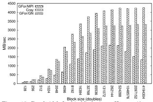
Figure 19: Bandwidth for big block sizes - Hopper 48 cores
