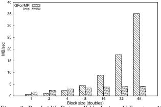
Figure 2: Bandwidth Put small block size - Yellowstone 16 cores
