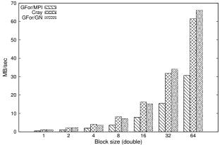
Figure 18: Bandwidth for small block sizes - Hopper 48 cores
