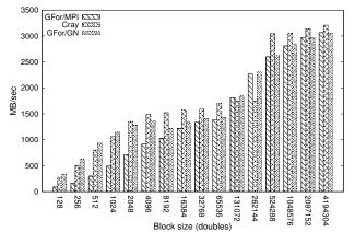
Figure 11: Bandwidth for big block sizes - Hopper 24 cores
