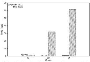
Figure 30: Distributed Transpose - GFortran vs. Intel
