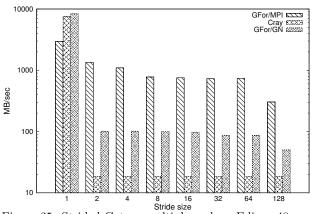
Figure 25: Strided Get on multiple nodes - Edison 48 cores
