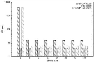
Figure 7: Strided Put on single node - Yellowstone 16 cores
