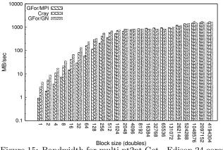
Figure 15: Bandwidth for multi pt2pt Get - Edison 24 cores
