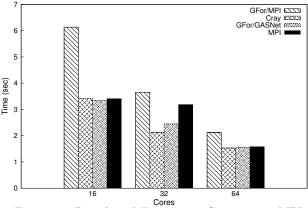
Figure 31: Distributed Transpose - Coarrays vs. MPI
