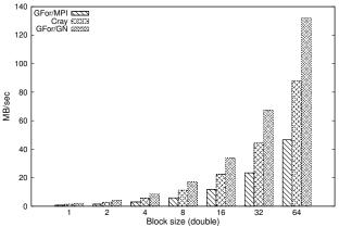
Figure 20: Bandwidth for small block sizes - Edison 48 cores
